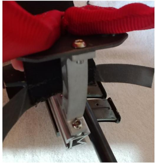
1-Place the pad on the rifle underneath the harness bracket with the hook & loop wings towards the bracket and start to wrap the wings around the sides of the bracket
