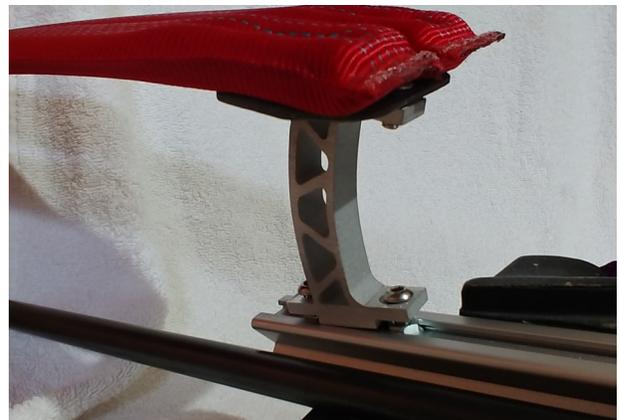
2-Slide the mounting bracket on to the rail ensuring that the shoulder straps are pointing up towards the barrel
