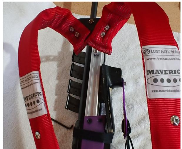
2-Adjust the angle of the shoulder straps to fit the athlete then tighten up all four screws
